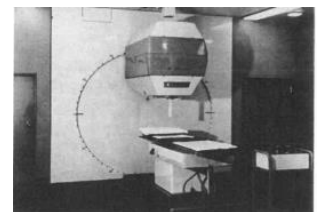
Toshiba 32 MeV Betatron at Kyoto
